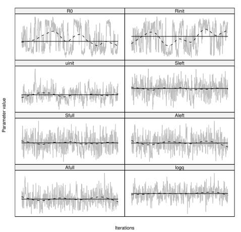
> plotTrace(xmcmc\$P, xlab="Iterations", ylab="Parameter value", layout=c(2,4))
