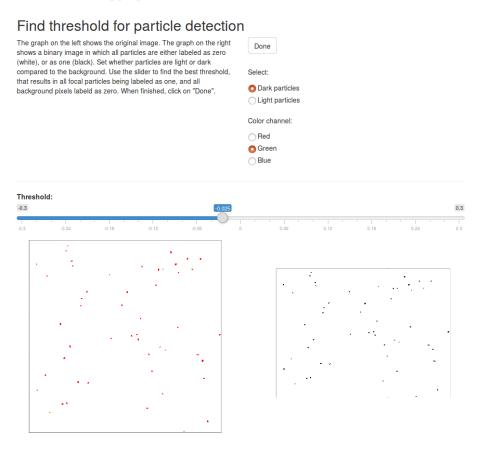
Figure 4: Graphical user interface to help users find the most appropriate threshold value.
